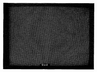
Figure 2-13 Color Purity Test
