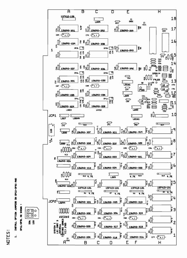
Figure 5-3 LSI Cartridge 3 PCB Assembly A043486-01 A
