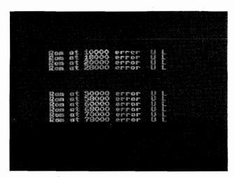
Figure 2-1 ROM Test Fails
