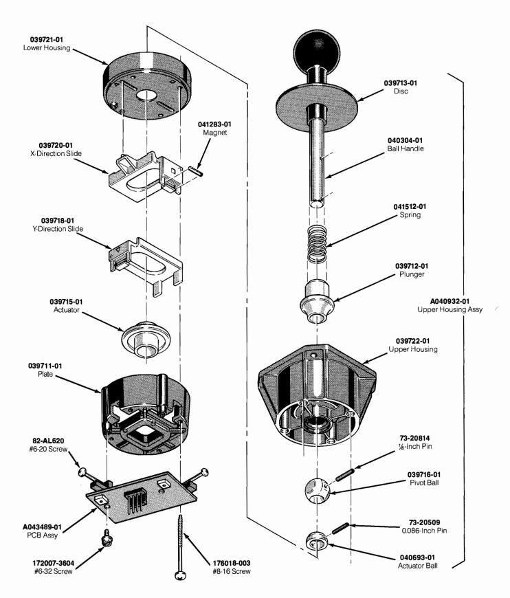
Figure 5-2 Hall-Effect Joystick Assembly A040935-01 D
