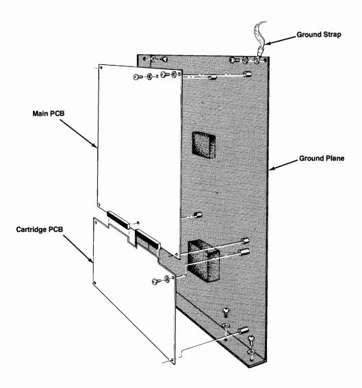
Figure 1-4 Cartridge PCB Replacement
