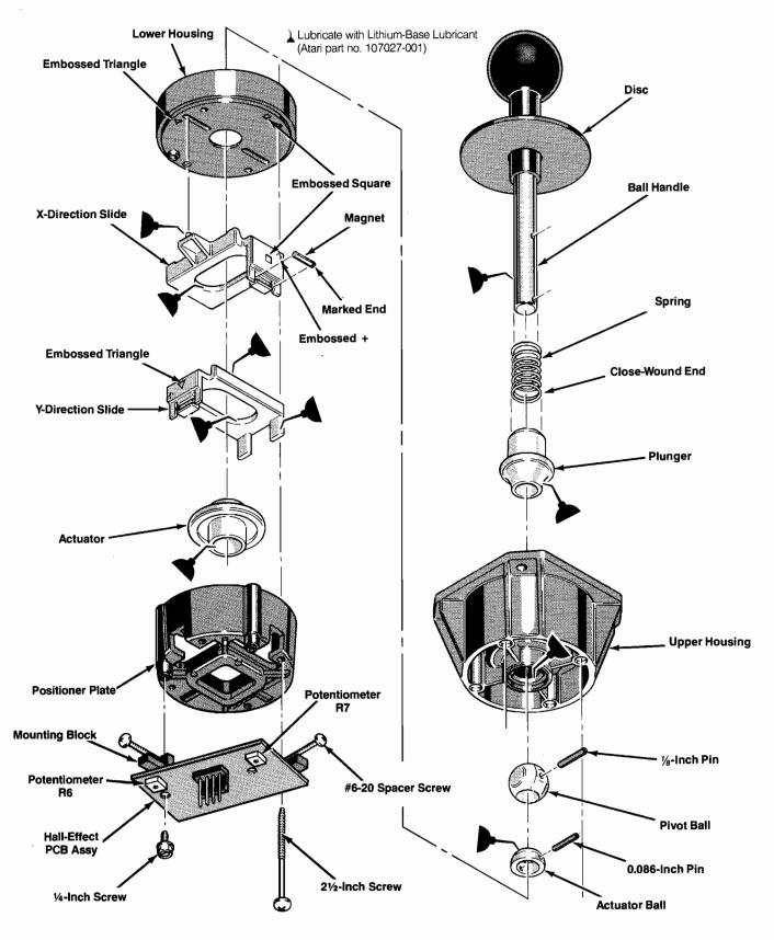
Figure 3-3 Joystick Disassembly and Lubrication
