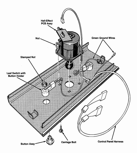
Figure 3-2 Removing the Joystick and Pushbutton Leaf Switches
