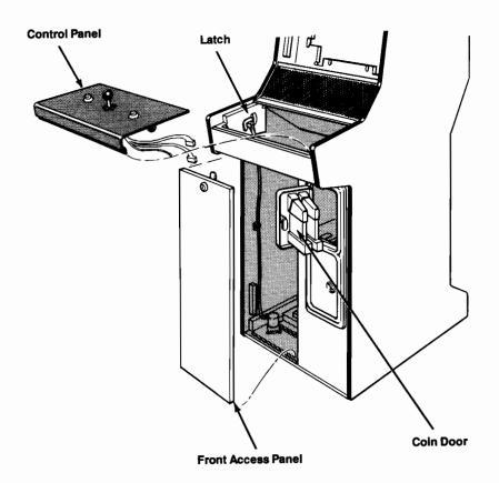
Figure 1-3 Control Panel Replacement
