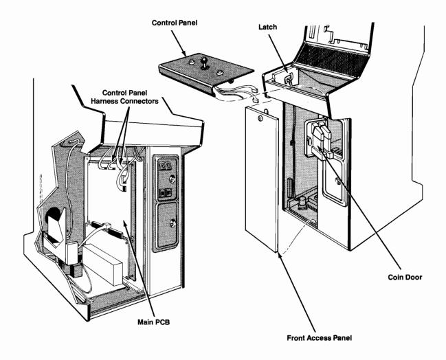
Figure 3-1 Removing the Control Panel
