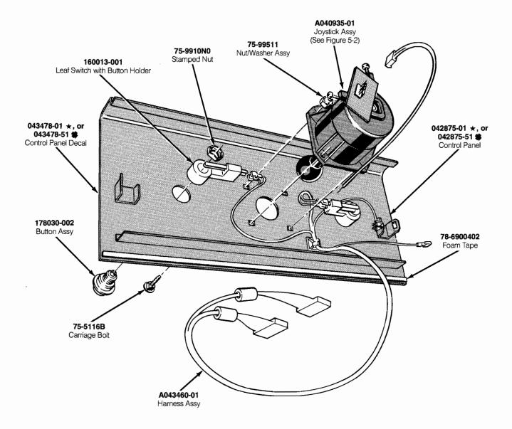
Figure 5-1 Control Panel Assembly A043477-01 A (US) and A043477-51 A (Ireland)
