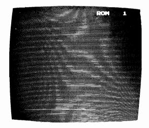
Figure 2-3 Self-Test Screen 1: Test Fails
