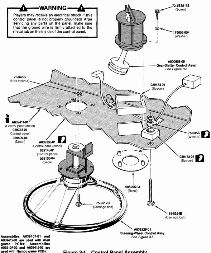
Figure 3-4 Control Panel Assembly Upright Cabinet A039412-01 & -02 A Sit-Down Cabinet A039107-01 & -02 B
