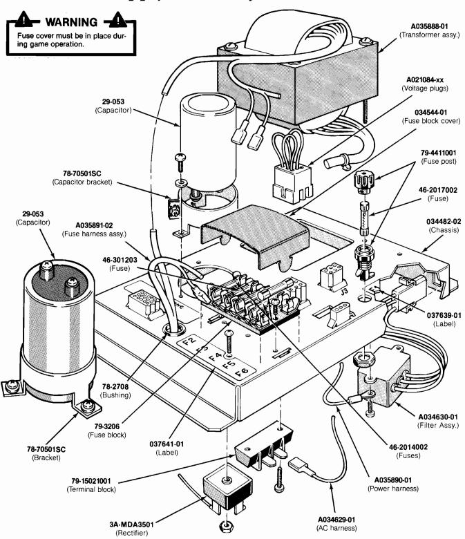
Figure 3-24 Power Supply Assembly A0376721-04 & -05 G
