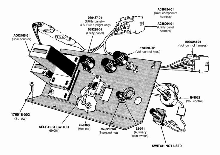
Figure 3-15 Utility Panel Assembly A039391-xx F
