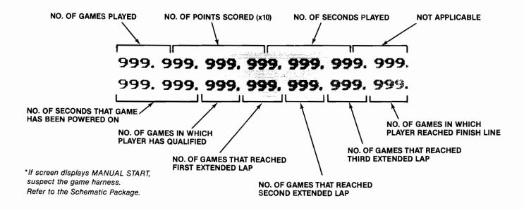
Figure 1-5 Self-Test Display
