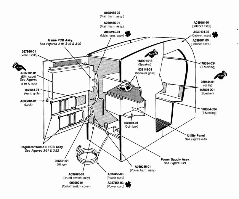
Figure 3-2 Cabinet-Mounted Assemblies U.S.-Built Sit-Down Cabinet A039100-01 F Ireland-Built Sit-Down Cabinet A039100-02 F
