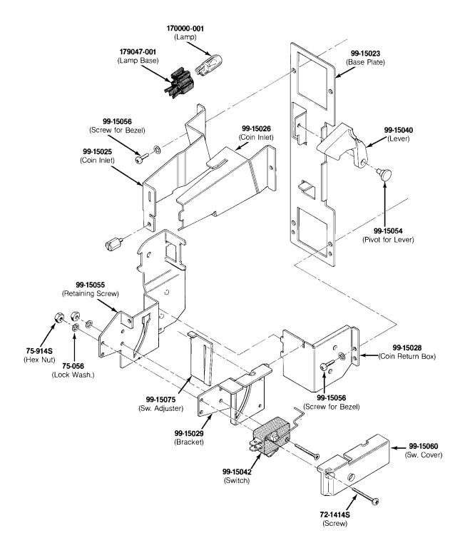
Figure 3-16 Vertically Mounted Coin Door 171034-xxx
