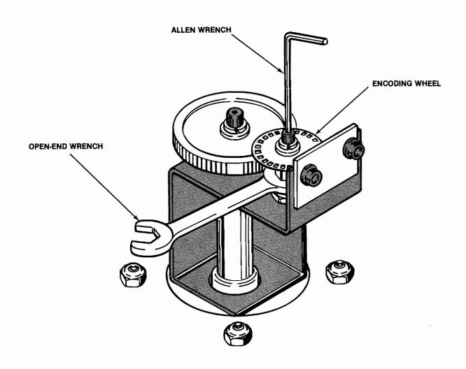
Figure 3-6 Steering-Wheel Control Screw Adjustment
