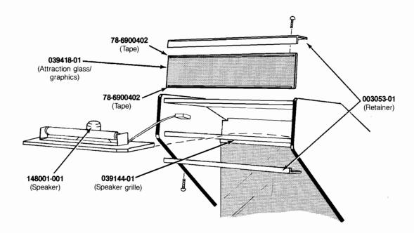
Figure 3-11 Fluorescent Tube and Speaker Board Removal Upright Cabinet
