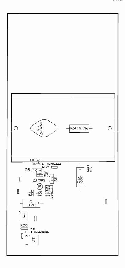
Figure 3-22 Regulator/Audio II PCB Assembly Ireland-Built Cabinet A035435-05 A
