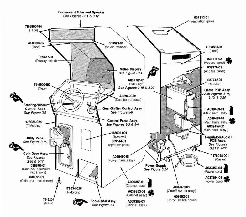
Figure 3-1 Cabinet-Mounted Assemblies U.S.-Built Upright Cabinet A039352-01 H Ireland-Built Upright Cabinet A039352-02 H
