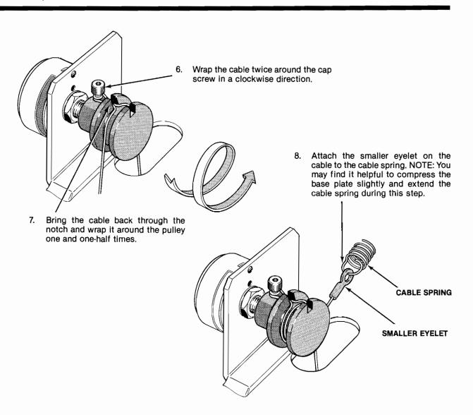
Figure 3-10 Foot-Pedal Pulley Cable Rewinding, continued
