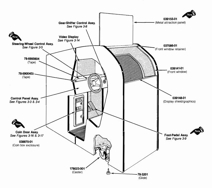
Figure 3-2 Cabinet-Mounted Assemblies, continued U.S.-Built Sit-Down Cabinet A039100-01 F Ireland-Built Sit-Down Cabinet A039100-02 F
