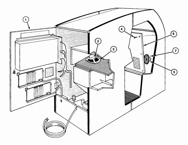
Figure 3-13 Sit-Down Cabinet Speaker Removal
