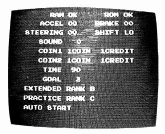
Figure 2-1 Self-Test Screen 1: Upright Test Passes
