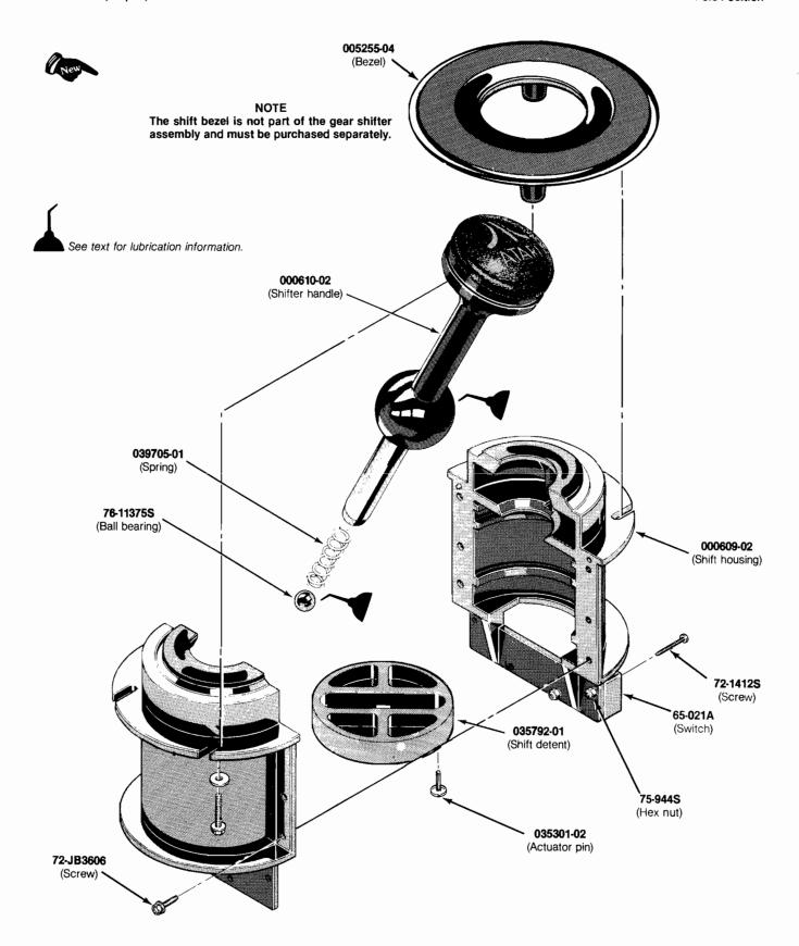
Figure 3-8 Gear-Shifter Control Assembly A000608-09 AB
