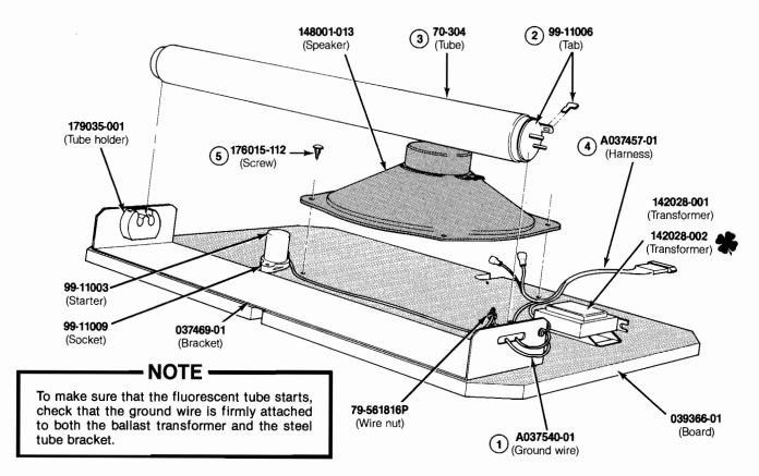
Figure 3-12 Fluorescent Tube and Speaker Board Assembly U.S.-Built Upright Cabinet A039415-01 A Ireland-Built Upright Cabinet A039415-02 A Parts List
