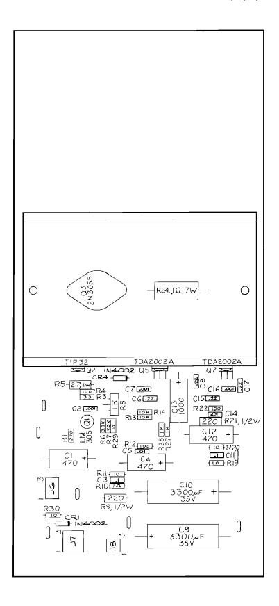
Figure 3-21 Regulator/Audio II PCB Assembly U.S.-Built Cabinet A035435-01 G
