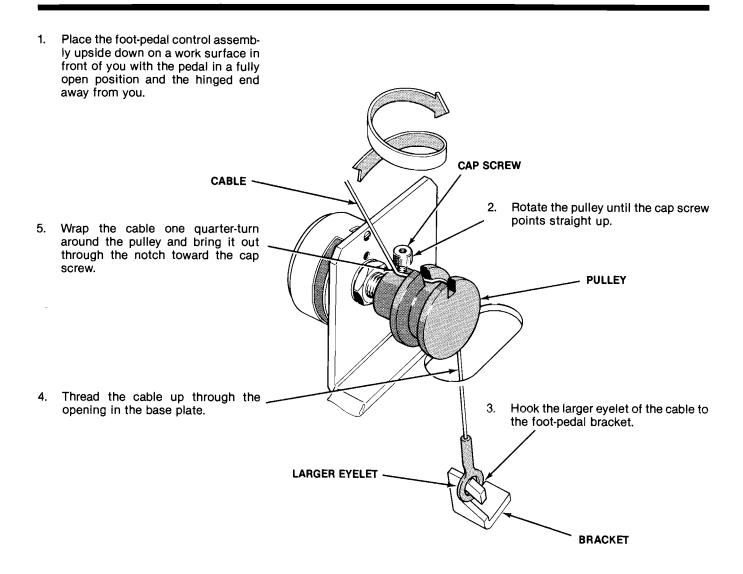
Figure 3-10 Foot-Pedal Pulley Cable Rewinding
