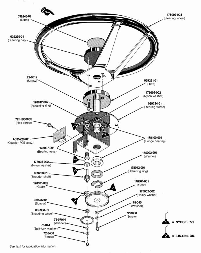
Figure 3-5 Steering-Wheel Control Assembly A039229-01 D
