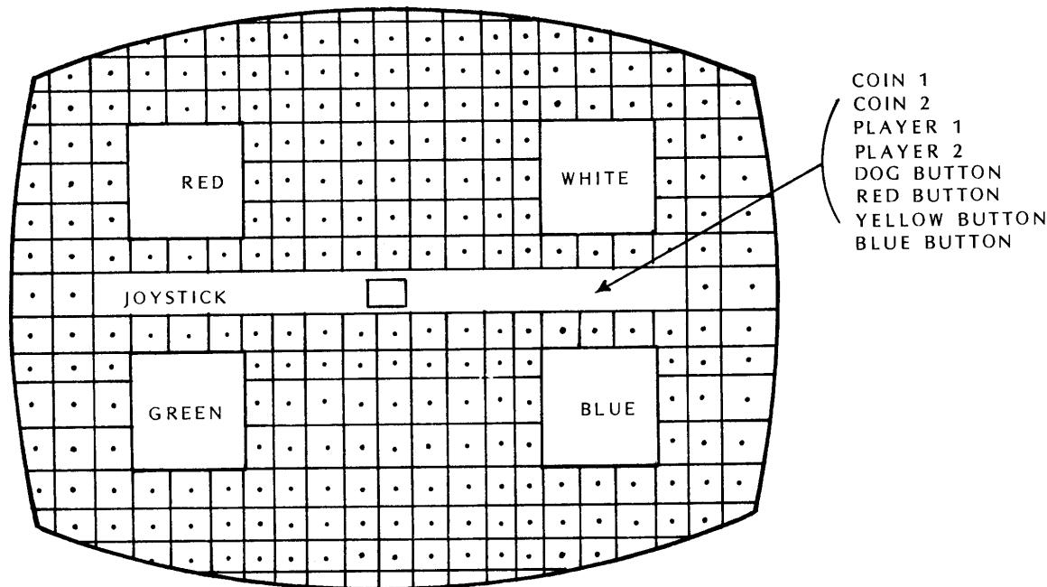
The grid pattern tests your screen for any distortion or convergence.
